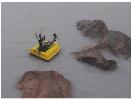
A sonar-equipped drone surveys Costa Rica's Laguna Catiente in the Poás volcano. The lake is 3 times more acidic than battery acid. Credit: David McFarlane
